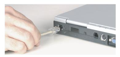
2. Insert the other end of the cable into a network jack (ask your network system administrator to help you select the correct network jack). Your Solo 3150 is now physically connected to the network. Your network system administrator can help you log on to establish an active network connection.
